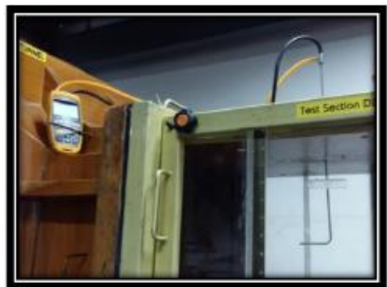
Fig 5: Pitot tube installation
