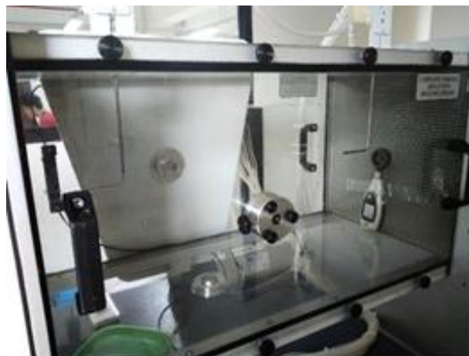
Figure 2. Anemometer inside the test section
