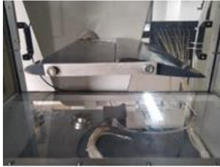
Figure 4. Tandem wing with NACA 0012 profile
