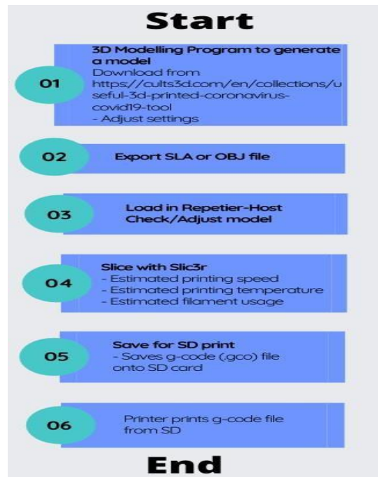
Figure 1: 3D printing face mask clips process
