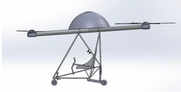
Figure 9: The center of gravity of the quadcopter
