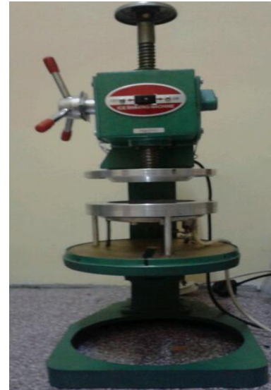
Fig. 13 - Prototype of Paper Plate Machine
