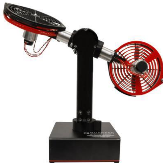
Figure 1: A 2-DOF helicopter model (Abdelkader and Kais, 2019)
