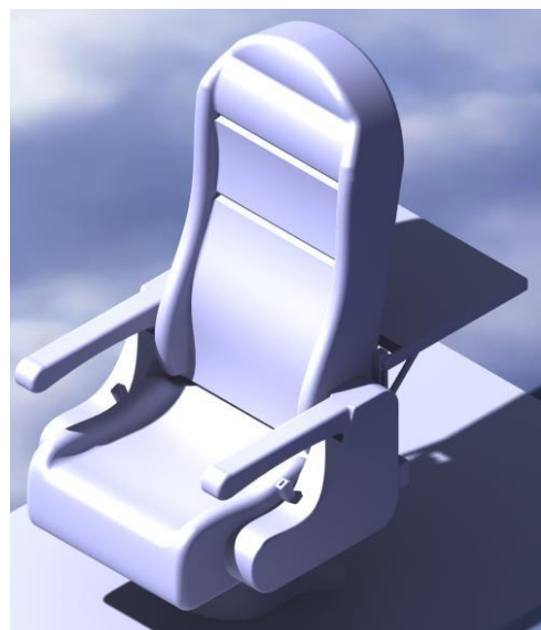
Figure2 - Complete model of new seat design in CATIA
