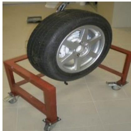
Figure 3 Unloaded condition tyre test setup
