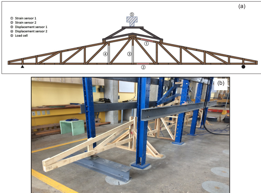
Figure 2 System for application of loads in truss tests (a) and restrictive elements used to avoid sideways motion of trusses during tests (b)
