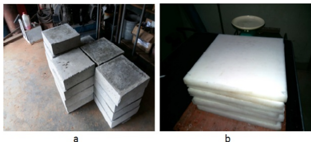
Fig.1 (a) K-500 concrete and (b) paraffin as shielding materials.
