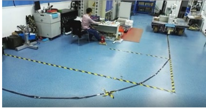
Figure 9. Straight-line tracking experiment process of omnidirectional AGV.
