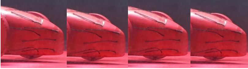
Figure 9: Wool tuft visualization on the front section of JM-5 model
