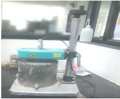
Fig. 2. Image of shrinkage meter.
